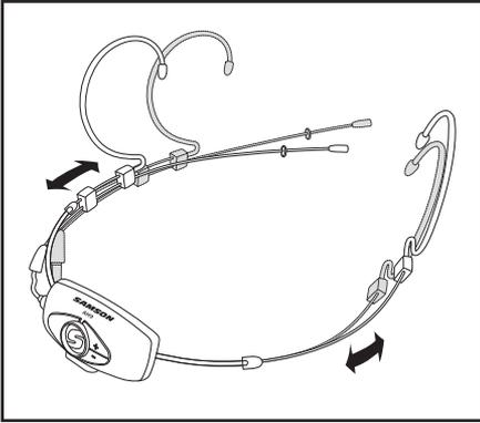
The DE10 headset can be sized by sliding the ear hooks to fit snug around your head. If the DE10 is loose and will not stay in place, slide the ear hook wires back for a tighter fit.
