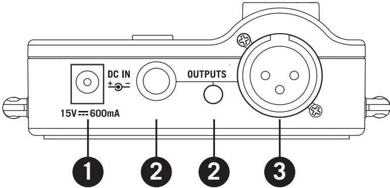
1. **DC Input** - Connect the supplied power adapter here.
