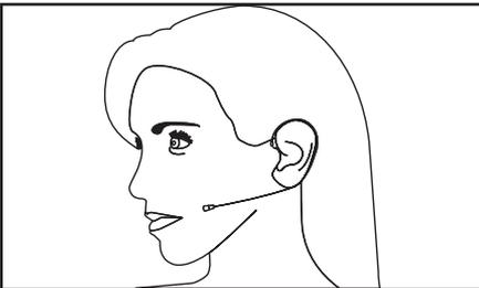
Position the DE10 microphone element about 0.25" – 1" behind the corner of your mouth. Since the DE10 is an omnidirectional capsule, the end of the microphone does not need to be facing your mouth. To avoid breath noise and p-pops, do not place the microphone directly in front of your mouth.
