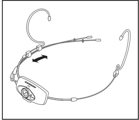
Adjust the microphone position by holding the left ear hook wire and slide the boom forward or back. For optimum performance the microphone should be close to the skin and towards the corner of the mouth, approximately a half inch away.
