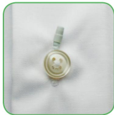
Ensure the entire cap of the B2D is exposed. Including small loops and taping the cable will help reduce handling noise.
