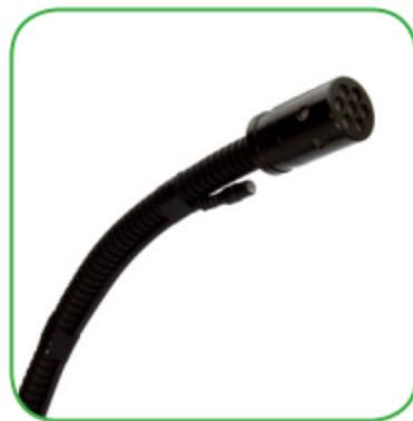
Black electrical tape holds the B2D under a podium microphone for redundancy. The technique also works well with omni B6 mics.
