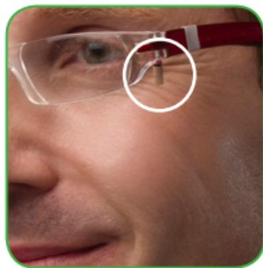
Heat shrink and a bent piece of wire hold the B2D in place. Point the capsule at the mouth (microphone extended for visibility).
