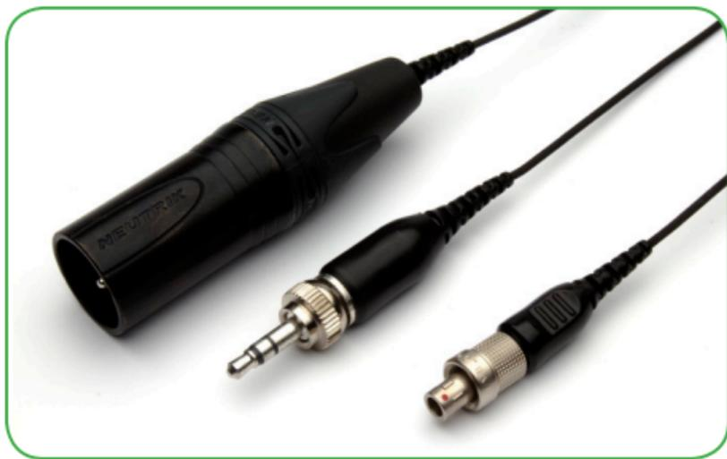
The B2D is available with threaded detachable connectors or permanently-attached connectors in a variety of configurations to suit hardwired systems and wireless transmitters. Make sure detachable connectors are firmly hand tightened before use. Both styles feature generous flex and strain reliefs bonded to Countryman's custom 1.5mm aramid-reinforced cable for more than 45 pounds of break strength.
